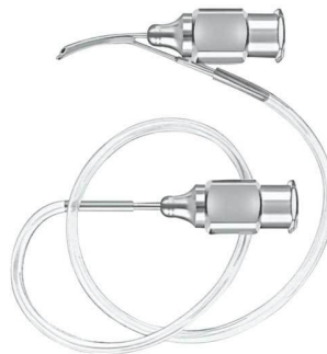
Item #: 4300 Name: SIMCOE I/A CANNULA CURVED Details: 15mm long, 0.3mm diameter aspiration port, front opening irrigation port, 23 gauge thin wall, for aspiration through tubing hub and irrigation through luer-lock hub
