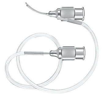
Item #: 4302 Name: Reversed Simcoe Irrigating-Aspirating Cannula Details: 15mm long, 0.3mm diameter aspiration port, front opening irrigation port, 23 gauge thin wall, for aspiration through luer-lock hub and irrigation through tubing hub
