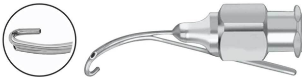
Item #: 4309 Name: Simcoe Irrigating-Aspirating Cannula Left Details: U-Shaped, 0.3mm anterior aspiration port, 23 gauge, supplied with silicone tubing and adaptor, for aspiration through tubing hub and irrigation through luer-lock hub
